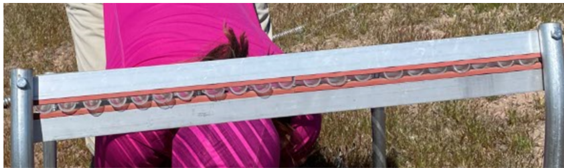
Figure A9.4. Images to help with rainfall structure construction. Note that there is no hardware keeping the roof slats in place, they are just squeezed between the metal pieces.
