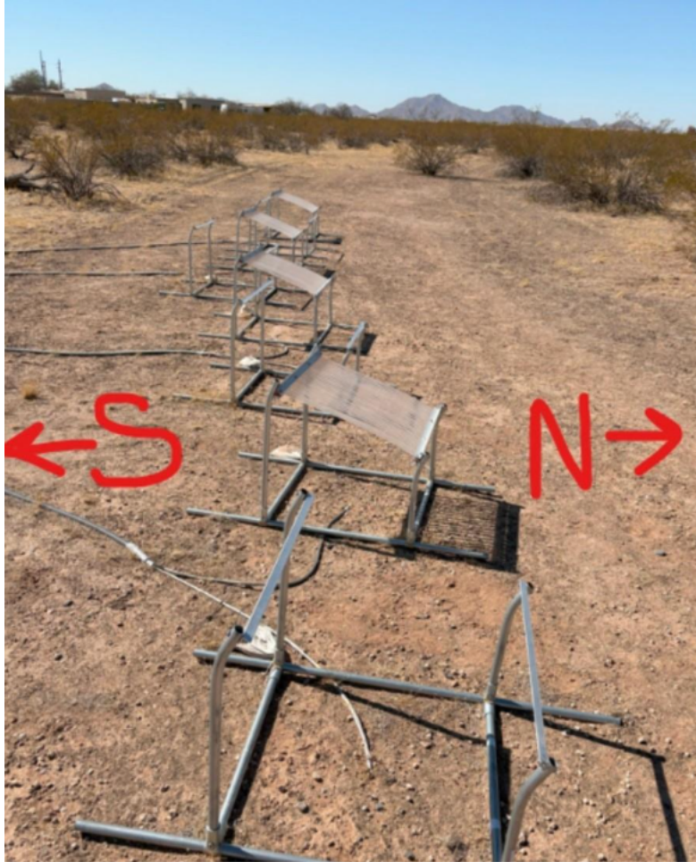
Figure A9.2. Shelter orientation with short legs facing north to minimize plot shading.
